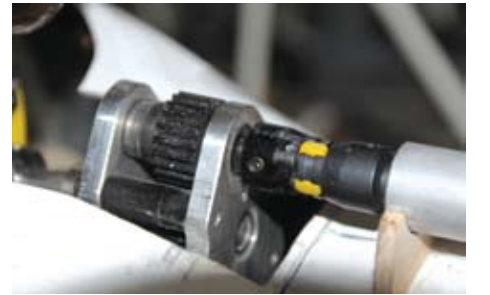
The intermediate gearbox positioned prior to finally being fixed in place
