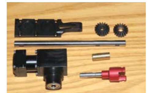
The tail gearbox components, notice the gearbox casing extension for the long output shaft
