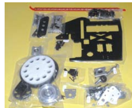
The mechanics parts are packed in numbered bags to coincide with the pages in the assembly manual
