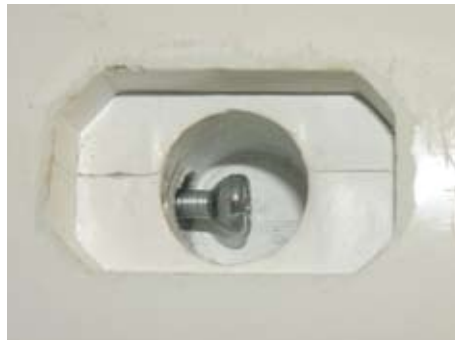
Here you can see the head of the cam bolt showing in the recess in the tail boom before the cam nut is fitted, plugs are provided to hide the recess
