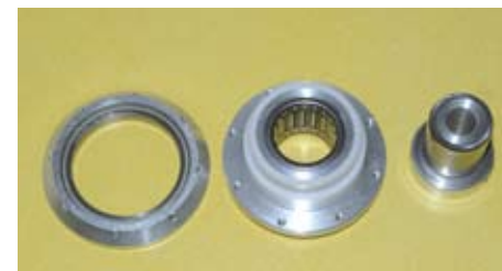
Here is the autorotation unit; it depends on which way this is assembled in the mechanics that dictates the rotation of the rotor head
