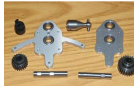
Component parts of the intermediate gearbox before assembly
