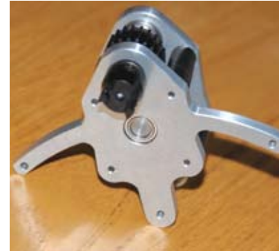
Intermediate gearbox assembled prior to fitting in the fuselage
