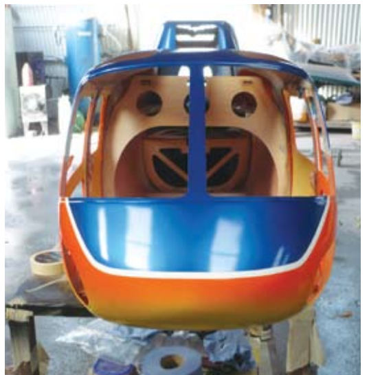
Looking into the front of the fuselage you can see the front former that the mechanics are anchored to and the rear formers that stiffen the rear section of the fuselage
