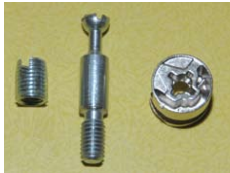
Here we have the screw insert cam bolt and cam lock nut, four of these hold the tail boom in place
