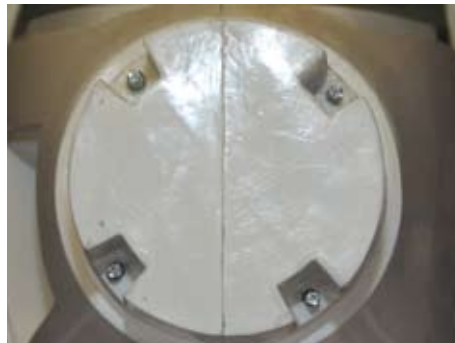
The four cam bolts are installed in the cutouts in the rear of the front half of the fuselage
