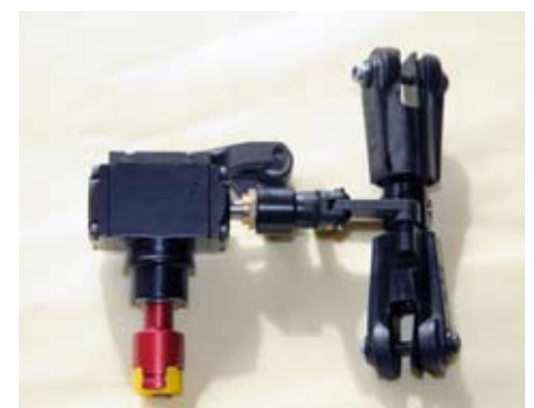
The tail gearbox will again be a familiar unit for any one who has built a large Vario machine
