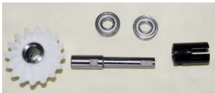
The components that make up the tail output, the large bevel gear takes the drive from the layshaft
