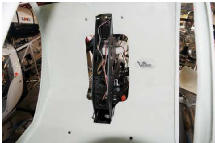
The cabin is held in place by four cap screws in addition to the valance beneath the front
