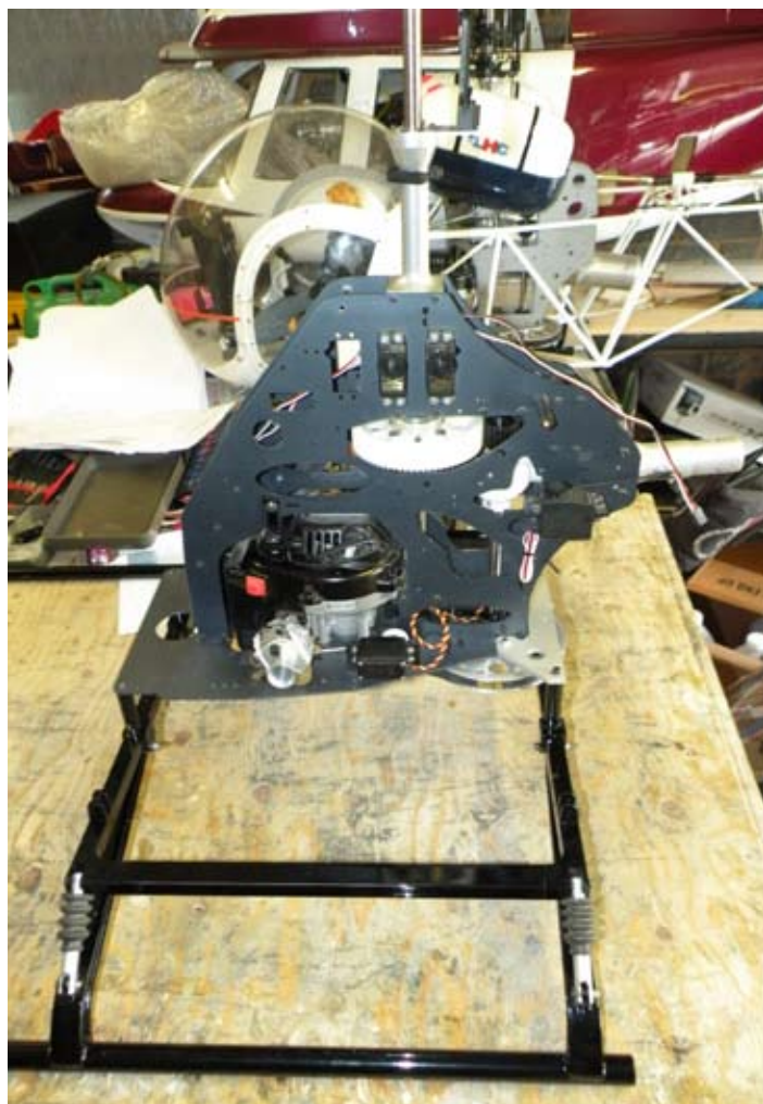
Standing on its own two feet so to speak, the mechanics are attached to the undercarriage frame
