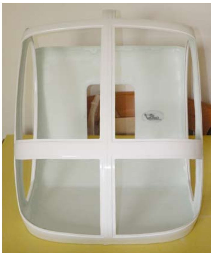
With the windows and doors cut out you can mount the cabin onto the mechanics
