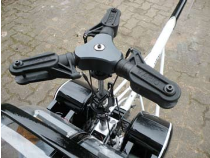
The rotor head has a metal centre block with composite grips; you can also see the frames that carry the fuel tanks attached to the back of the cabin
