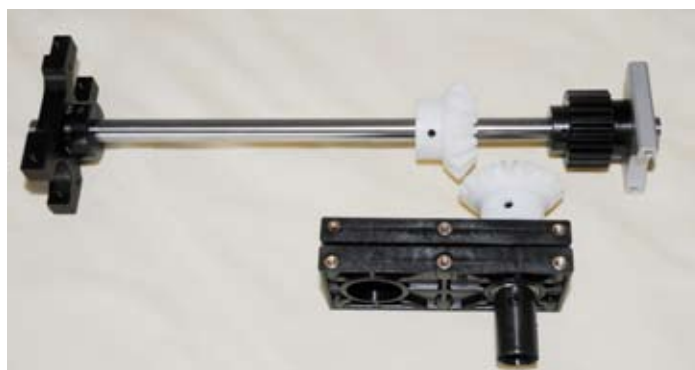
The components that make up the tail output, the large bevel gear takes the drive from the layshaft
