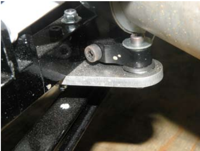
The exhaust pipe is securely held in place by this cleverly designed rubber mounted clamp
