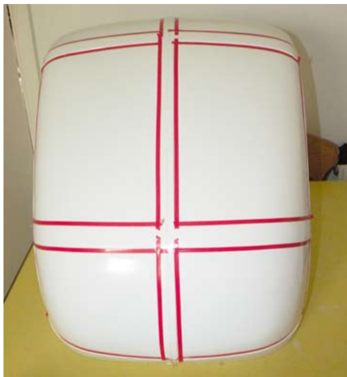
I always use 6 mm wide tape to mark where the windows need to be cut; this leaves a lip for the glass to sit on
