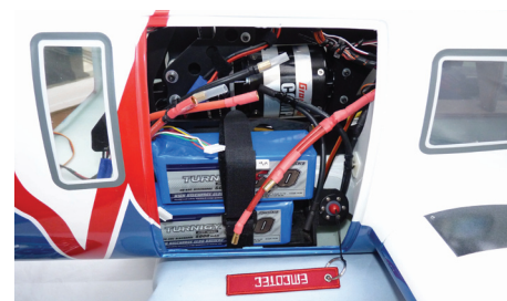
Two 5000 mAh 6S LiPo's connected in parallel are fitted each side and connected in series to power the model, see text for details of the wiring pull the red Emcotec plug and the system is live
