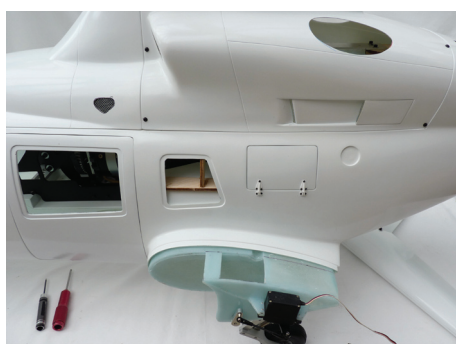
Access panel hides a board for switches etc. – not used in this electric version; the main side door is retained with magnets
