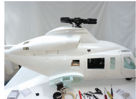
Top cowls fit really well, here the doors have been fitted, the front ones are hinged while the rear are held in place with magnets
