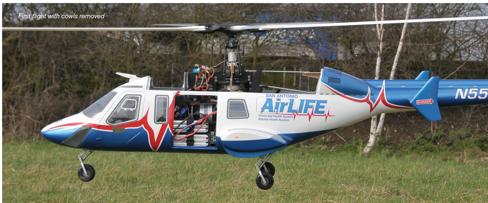
Two 5000 mAh 6S LiPo's connected in parallel are fitted each side and connected in series to power the model, see text for details of the wiring pull the red Emcotec plug and the system is live
