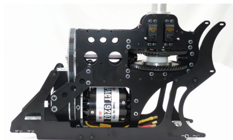
Here the lower frames have been added and it's ready to go into the fuselage
