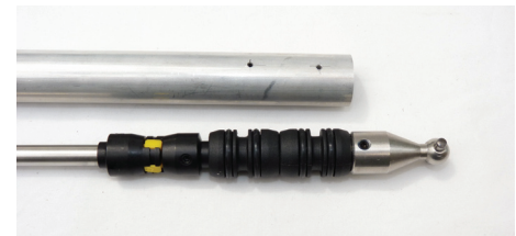
The front section of the tube drive is strongly supported because the section to the mechanics is unsupported
