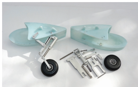
These are the side pods and super retract system, I had to rework the axle holes in the pods – see text for details
