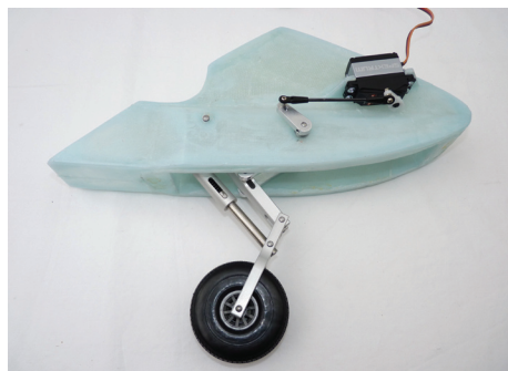
This is the nose wheel pod and you can see the oleo, the weight of the model means the oleo bottoms so the model is stable on the ground
