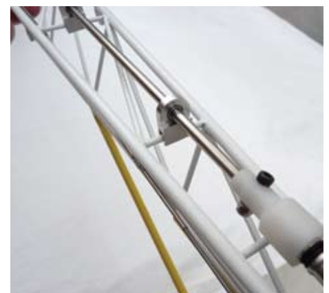
Very neat bearing holders for the tail drive tube; you can just see the 'O' rings that are used to limit the end float
