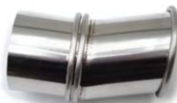
The exhaust extension is not necessary but looks the part and deflects the hot exhaust away from the tail
