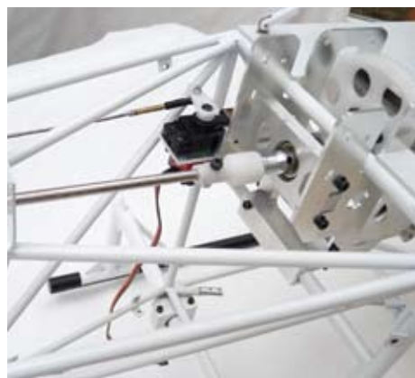
Tail drive is very simple; here you can see the tail servo and the control rod
