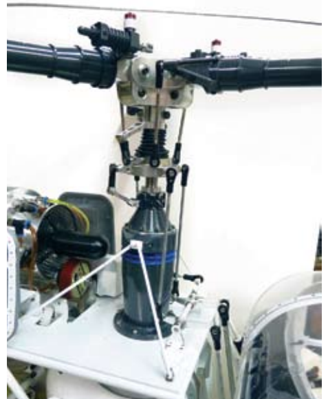
See the swashplate is offset by 45°; I have positioned the inner ring such that the pitch rods are vertical and phasing is electronically corrected
