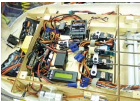
Revised layout, the HeliCommand HC3-Xtreme is between the servos that now have 20 mm arms, the yellow box is the electronic switch for the lights
