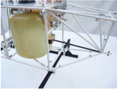
This shows the carbon tube brace that holds the tank forward...
