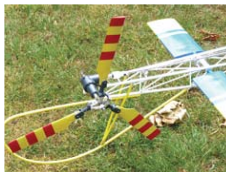
I used extra coats of lacquer to balance the painted tail blades
