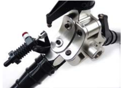
The blade grips pivot about the upper pin, while the lower pin is damped
