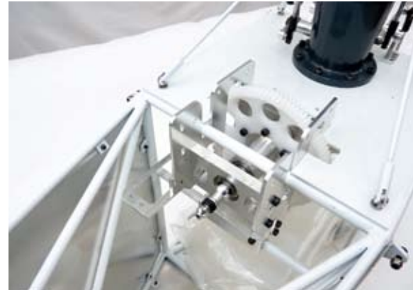
Here is the layshaft with the spur gear mounted on the auto unit
