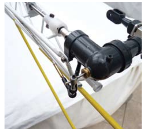
The tail pitch change rod connects to an actuation lever that rotates about a fixed link, thus as the lever is pulled/pushed, it moves the pitch rod
