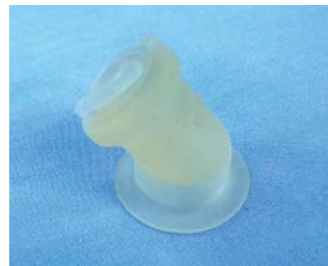
The scale fuel filler was produced using a 3D printer and adds to the finished model
