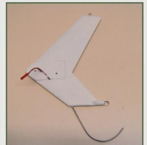
Stabiliser modified with anti-collision light and tail skid, which was later shortened
