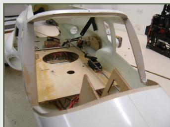
Preparing the fuselage window section for a removable frame to enable easy change of batteries
