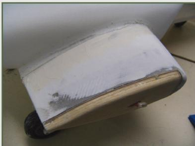
Wing stubs with retractable wooden frame. Inside are the cables for the positioning lights and target acquisition LEDs
