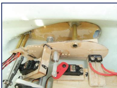
**Right: Servo assemblies for retractable gun frame and extendable guns**
