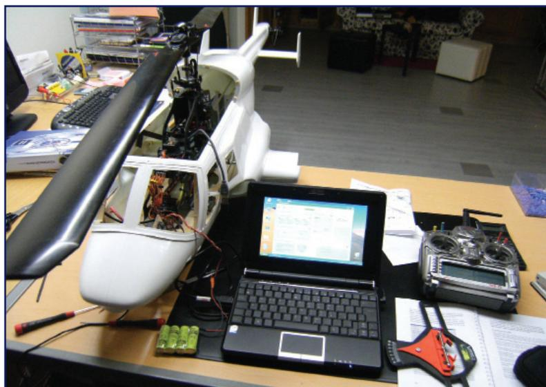
**Programming the transmitter and flybarless system with a laptop computer**
