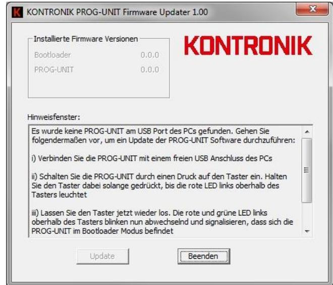
Press the button on the backside of the ProgUNIT and hold it during the following steps. Connect the USB port of the ProgUNIT with the included USB cable to your PC. The green LED is shining. Wait and still **hold the button pressed** until the red LED begins to shine also . This procedure may take up to six seconds. After the red LED begins to shine, release the button and both LEDs will flash alternately.
