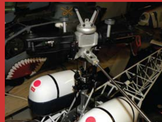
The scale rotorhead has a dummy Bell Bar, and so flies as a flybarless rotorhead.
