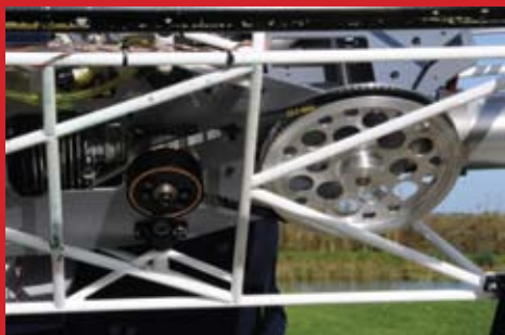
Drive is taken from the clutch to the mechanics by a toothed belt and this large pulley is simple and efficient
