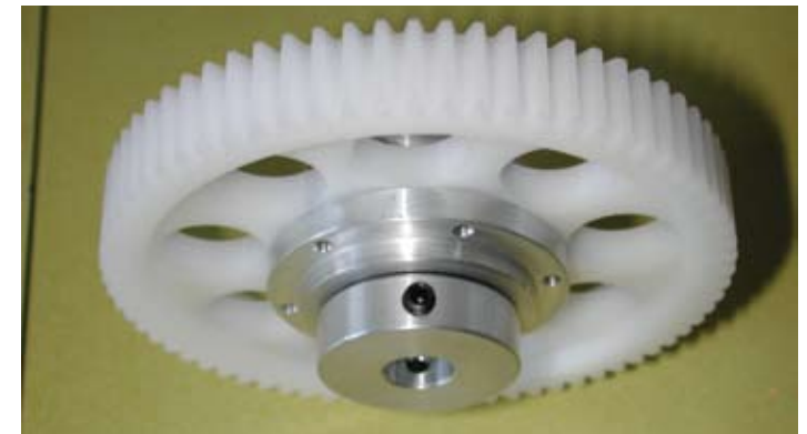
This sturdy main gear has the autorotation unit attached and is clamped to the main shaft by the visible grub screw
