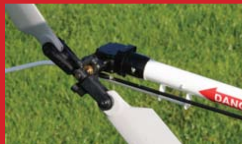
ABOVE: The flybar rotor head makes the model fly how I like it
