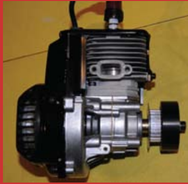
The trusty Zenoah G230 petrol engine is certainly powerful enough and reliable
