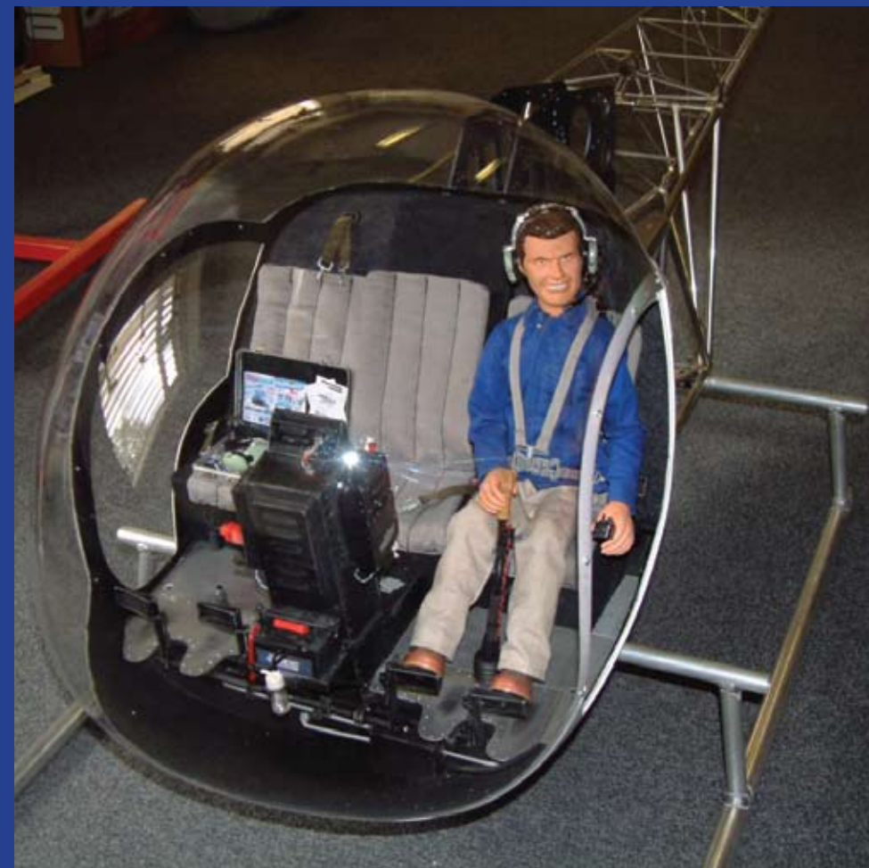
John White's beautifully crafted Bell 47 scale cockpit, the pedals, cyclic stick and collective lever all move following the Tx control and the pilot's head rotates with yaw control
