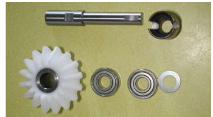
The tail drive is transmitted through this bevel gear, which as you can see this is more than strong enough
