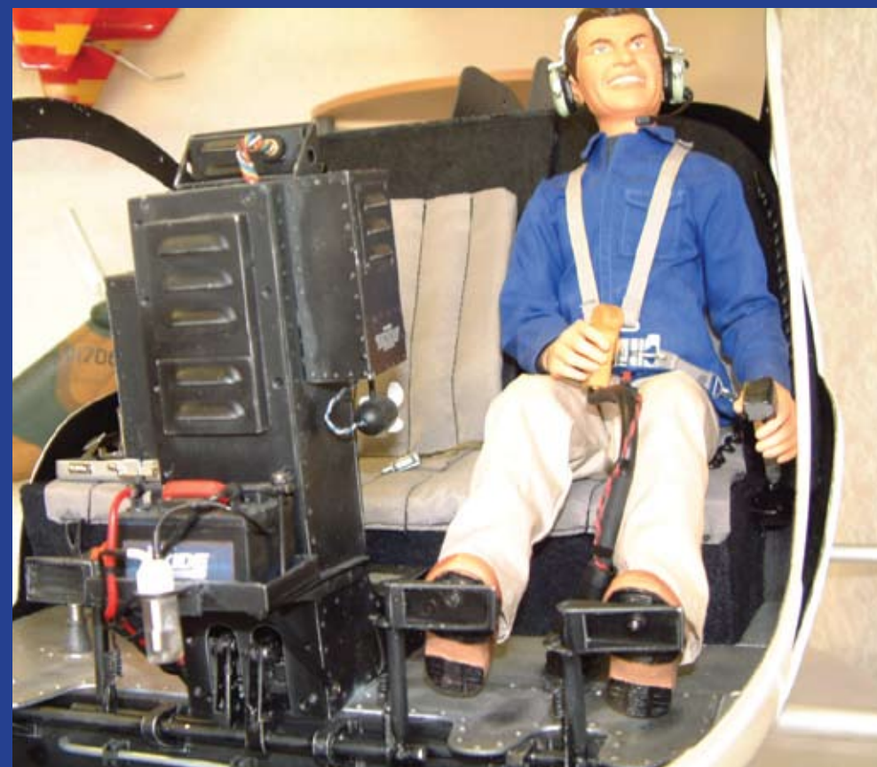
John White's beautifully crafted Bell 47 scale cockpit, the pedals, cyclic stick and collective lever all move following the Tx control and the pilot's head rotates with yaw control
