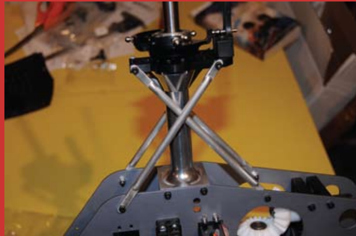
This metal mast support with braces is added because the main shaft is 514 mm long!
