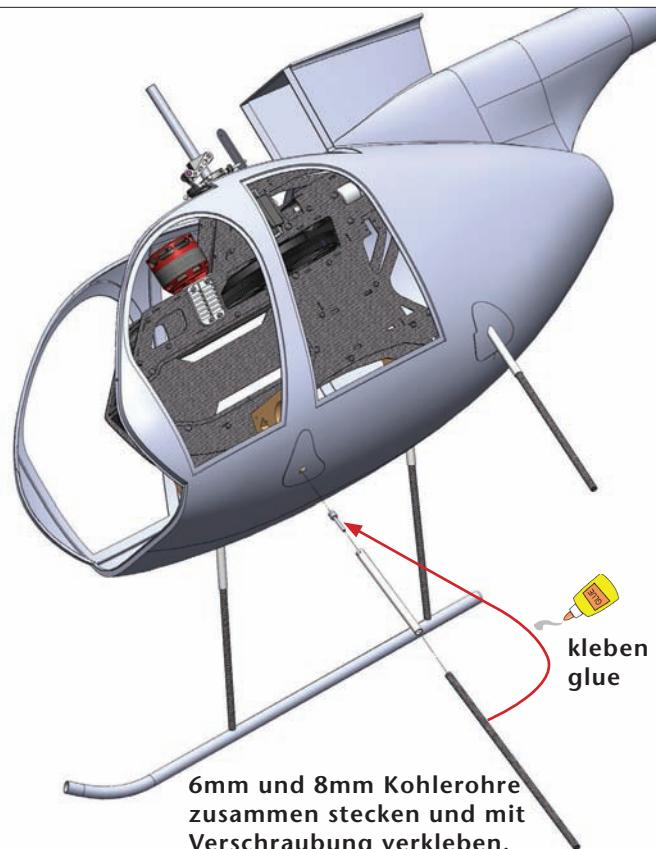
slide 6mm tube inside 8mm tube, glue threaded aluminium part
